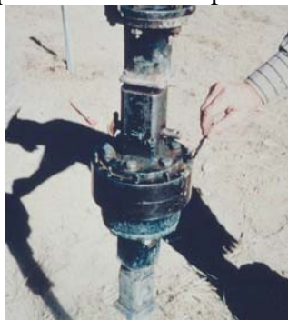
Photo 9-11 Shear-pin torque indicator.
