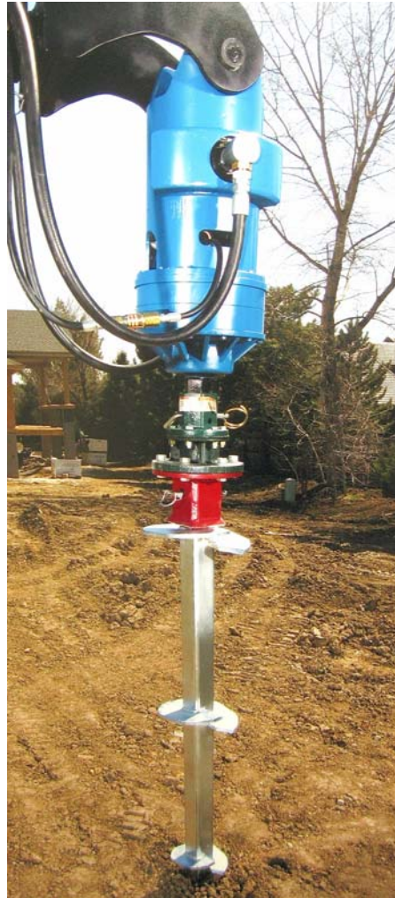
Photo 8-1 Helical pile drive head with kelly bar adapter and drive tool.
