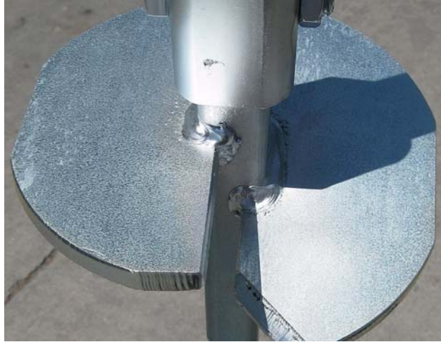
Photo 9-10 Helix welded to the central shaft
