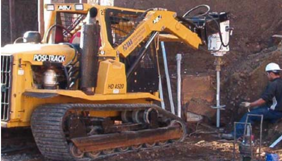
Photo 1-53 This tracked installation machine is ideal in tight access locations and wide open spaces.
