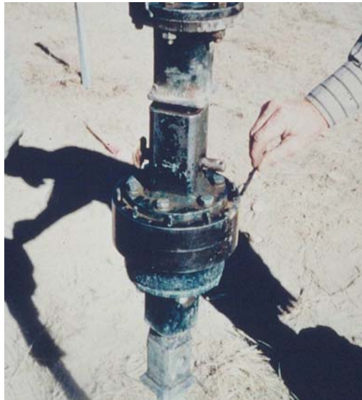
Photo 2-1 Shear Pin Torque Indicator
