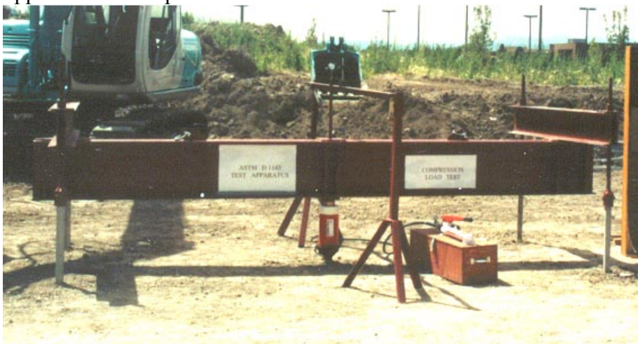
Photo 3-1 Compression load test set-up for helical pile.
